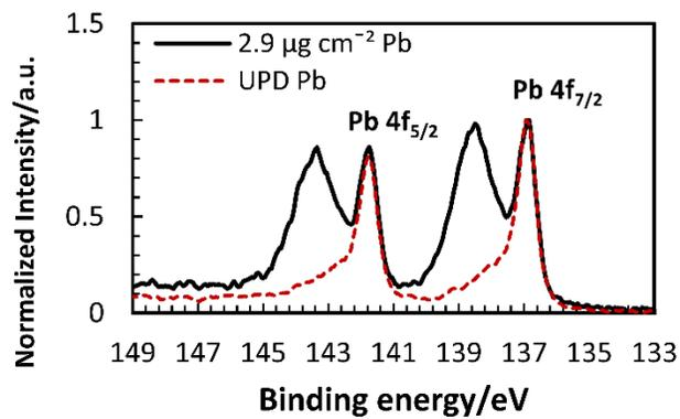
**Fig. 2.** Normalized Pb 4f X-ray photoelectron spectra for a sample with  $2.9 \mu\text{g cm}^{-2}$  Pb added during electrolysis and a sample with Pb deposited by UPD. The peaks at 143.4 eV and 138.4 eV are indicative of  $\text{Pb}(\text{OH})_2$ , which is believed to have formed after the experiment.
