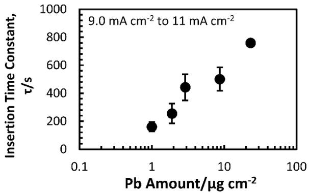
**Fig. 4.** Insertion time constant,  $\tau$  vs Pb amount for the  $-9.0 \text{ mA cm}^{-2}$  to  $-11 \text{ mA cm}^{-2}$  step. More Pb increases the amount of time required to reach a steady-state hydrogen content.
